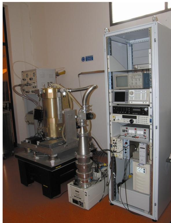
**Fig. 2.** The cryostat used for developing low temperature detectors.
