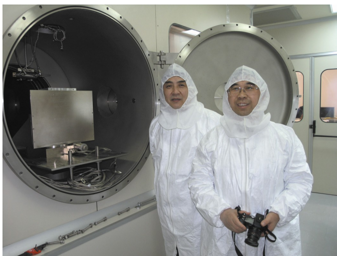
Inside the clean room, during the installation of the LOXIA detector for the Chinese CHANG'E1 mission in the vacuum chamber.
